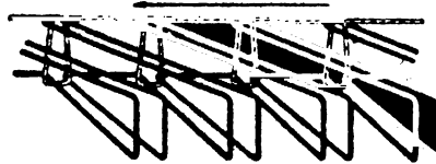
FIG. 30 TWO-THREAD OVERLOCK STITCH
